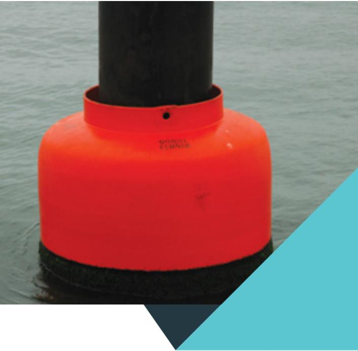
Donut Fenders are the perfect choice for tidal zones berthing. The donut floats around a tubular pile which is easy to install and follows changes in the water level. It uses the same technology as Foam Filled Fenders with closed-cell polyethylene foam core to absorb impact and tough enough polyurethane elastomer to resist wear and tear. The Donut's durable low-friction bearings allow free movement with minimal maintenance.
