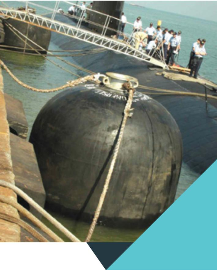
Fender Marine Hydro-Pneumatic Fenders make contact with vessels such as submarines below the water-line. Hydro-Pneumatic Fenders also can be used for vessel-to-vessel. Fenders are part-filled with water and ballasted to float vertically. Performance can be tuned by changing the water-to-air ratio and initial pressure.
