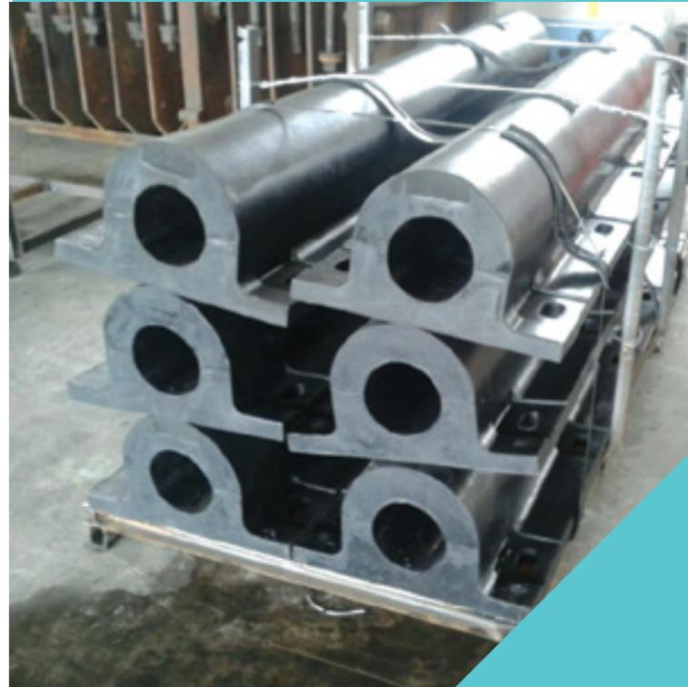
Wing Fenders are usually used for tugs and workboats. Instead of drilling the fender, the wings of the Wing Fender are retained by steel angles. Wing Fenders are jacked into the angles during installation and joints between adjacent sections are "plugged" to achieve a smooth and continuous contact face. Once fitted, the "wings" of the Wing Fender sit tightly within the angles making this arrangement very resistant to longitudinal and transverse shear.
