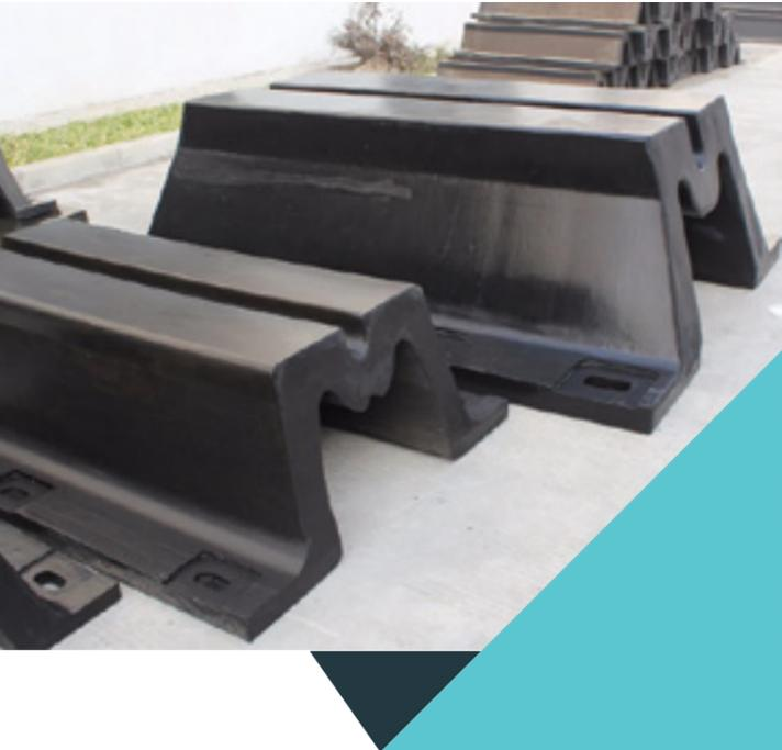
M Fenders have a low weight per contact area. They can be fitted around very tight curves, fixed with pins that run through central bore holes. They are grooved for a soft and flexible contact face, which firmly grips the vessel's hull.
